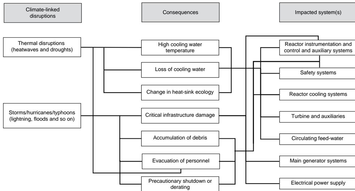
**Fig. 1 | Pathways of climate-induced disruptions in nuclear power plants.** This figure maps climate-linked disruptions and their respective consequences to the specific reactor system they impact. Each pathway is a potential route of a partial or full reactor outage.
