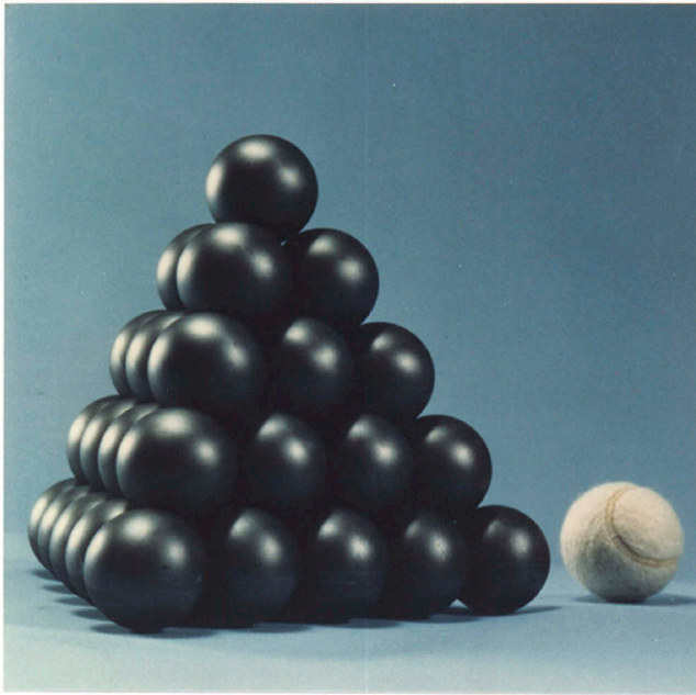
Figure 1. In pebble reactors, the fuel consists of small (roughly 6 cm in diameter) uranium particles, coated with several ceramic layers and graphite.
